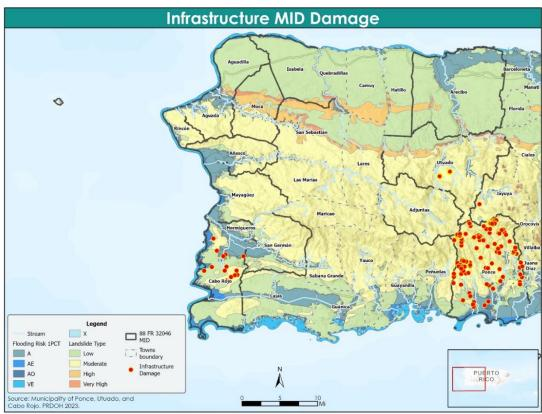
Figure 36: Infrastructure MID Damage. Red dots identifying locations of documented damages in the Municipalities of Utuado, Cabo Rojo, and Ponce.
